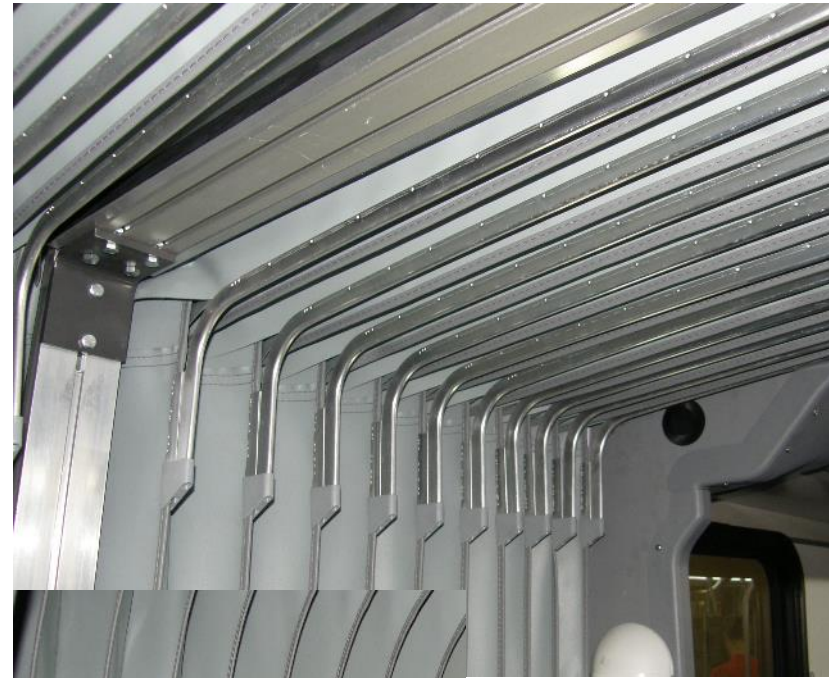
False ceiling mount with solid plastic clip screwed to support extrusion
