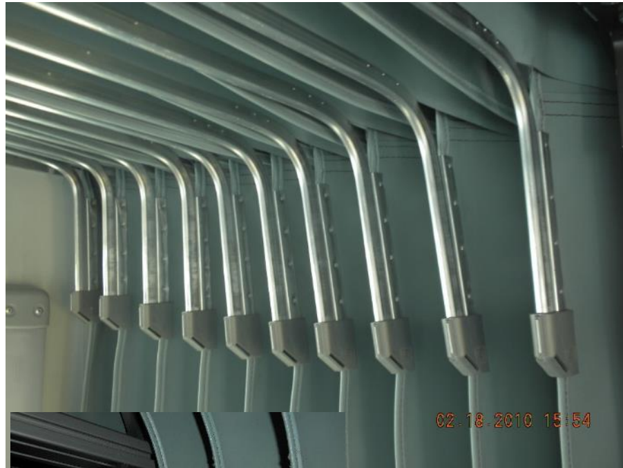
False ceiling mount with folding plastic clip
